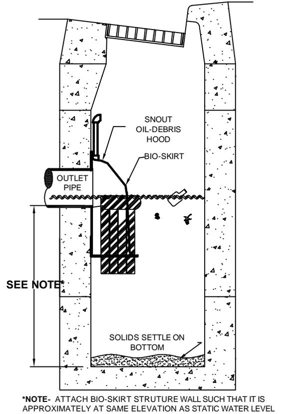
\*NOTE- ATTACH BIO-SKIRT STRUTURE WALL SUCH THAT IT IS APPROXIMATELY AT SAME ELEVATION AS STATIC WATER LEVEL
