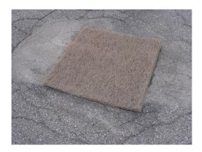
Coir Inlet Mat shall be applied as a storm water silt filter at sewer inlets. Cut the mat to allow 3" overlap at each side of the grate. Attach the mat to the topside of the inlet grate using wire or plastic ties. Clean silt from Coir Inlet Mat and surrounding area following each rainfall.
