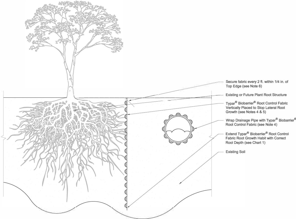
**Biobarrier® : Drain Line Application**
