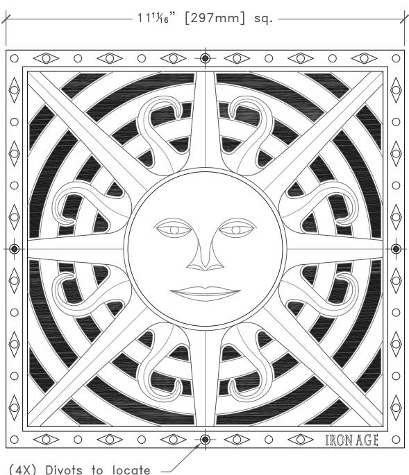
(4X) Divots to locate bolt—down holes as desired
