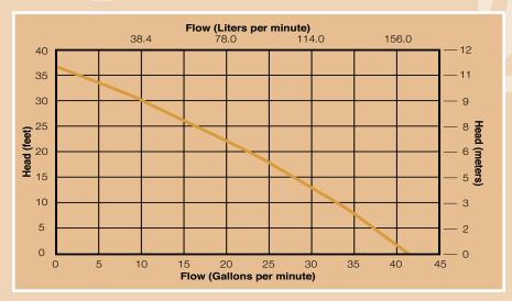
**Note:** Maximum shut-off head is 36 feet. Usable maximum head - assuming 150' of lateral discharge through 1" pipe is 25 feet. Consult factory for proper sizing and calculation of friction loss.
