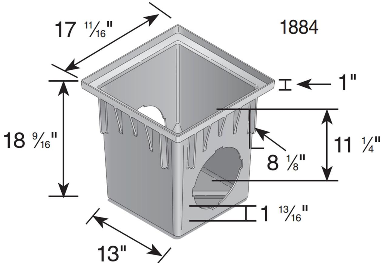
Material: UV Protected High Density Polyethylene (HDPE)
