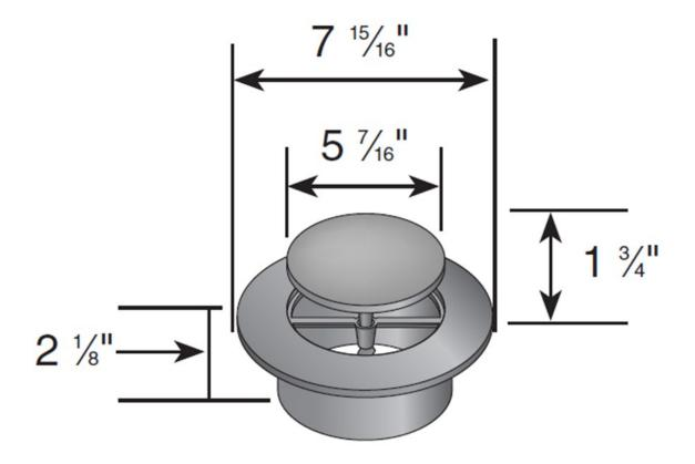
Part #: 620 Material: High Density Polypropylene (HDPE) Colors: Green Fits: 6" sewer and drain fittings and NDS 6" Spee-D Basin Spring: Stainless Steel Grade 302 Open Pressure: 1 PSI Open Surface Area: 28.8 Sq. Inches Flow Rate: 1" Head: 124.60 GPM 0.5" Head: 88.10 GPM Weight Per Each: 0.64 lbs. UV inhibitor
