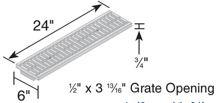
Material: UV Protected High Density Polyethylene
