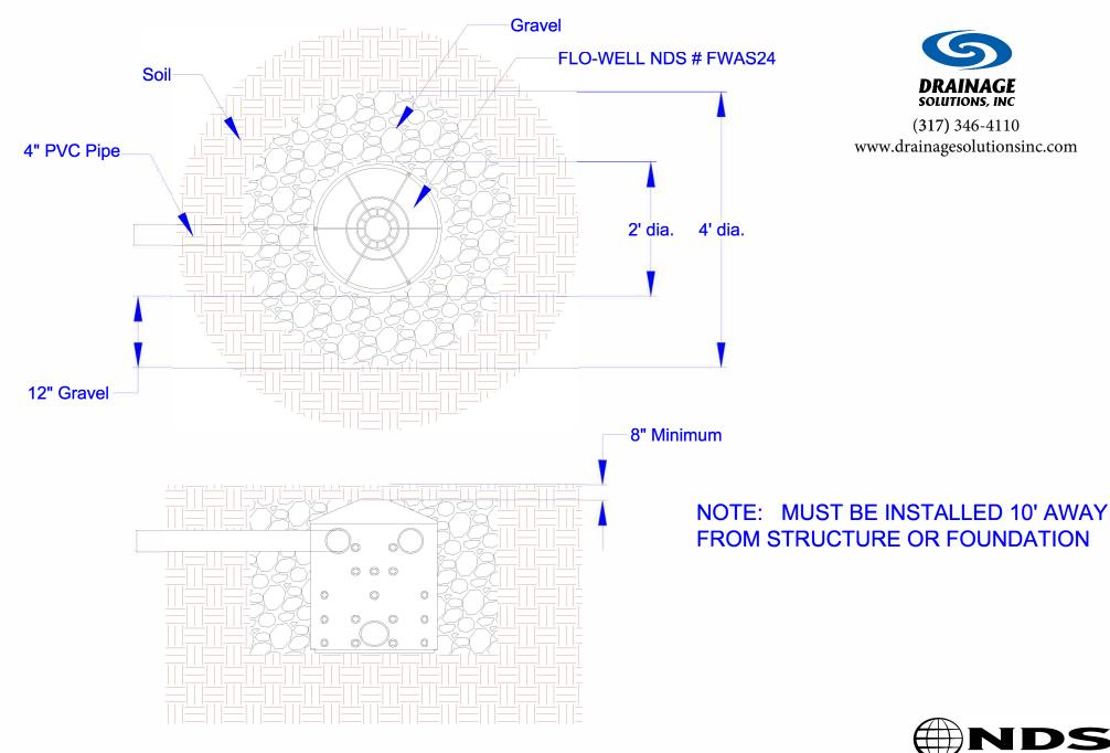
NDS Flo-Well Installation Detail in Gravel Backfill
