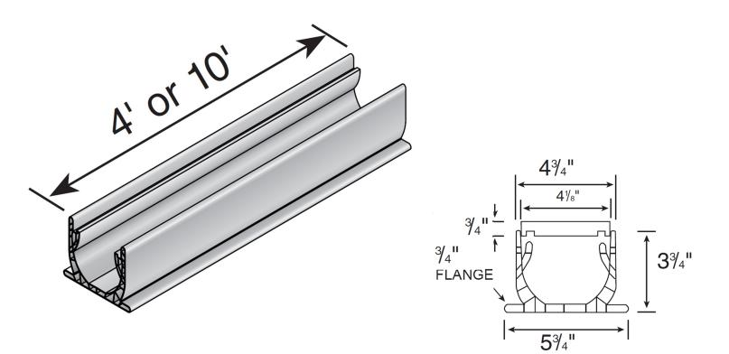
Part #: 400 ( 4 Ft.) , 400-10 ( 10 Ft.) Material: PVC Color: #400(Gray), and #400-10(Gray) Fits: 2" Sch. 40 pipe, 3" and 4" sewer and drain pipe with proper fittings. UV Inhibitors.
