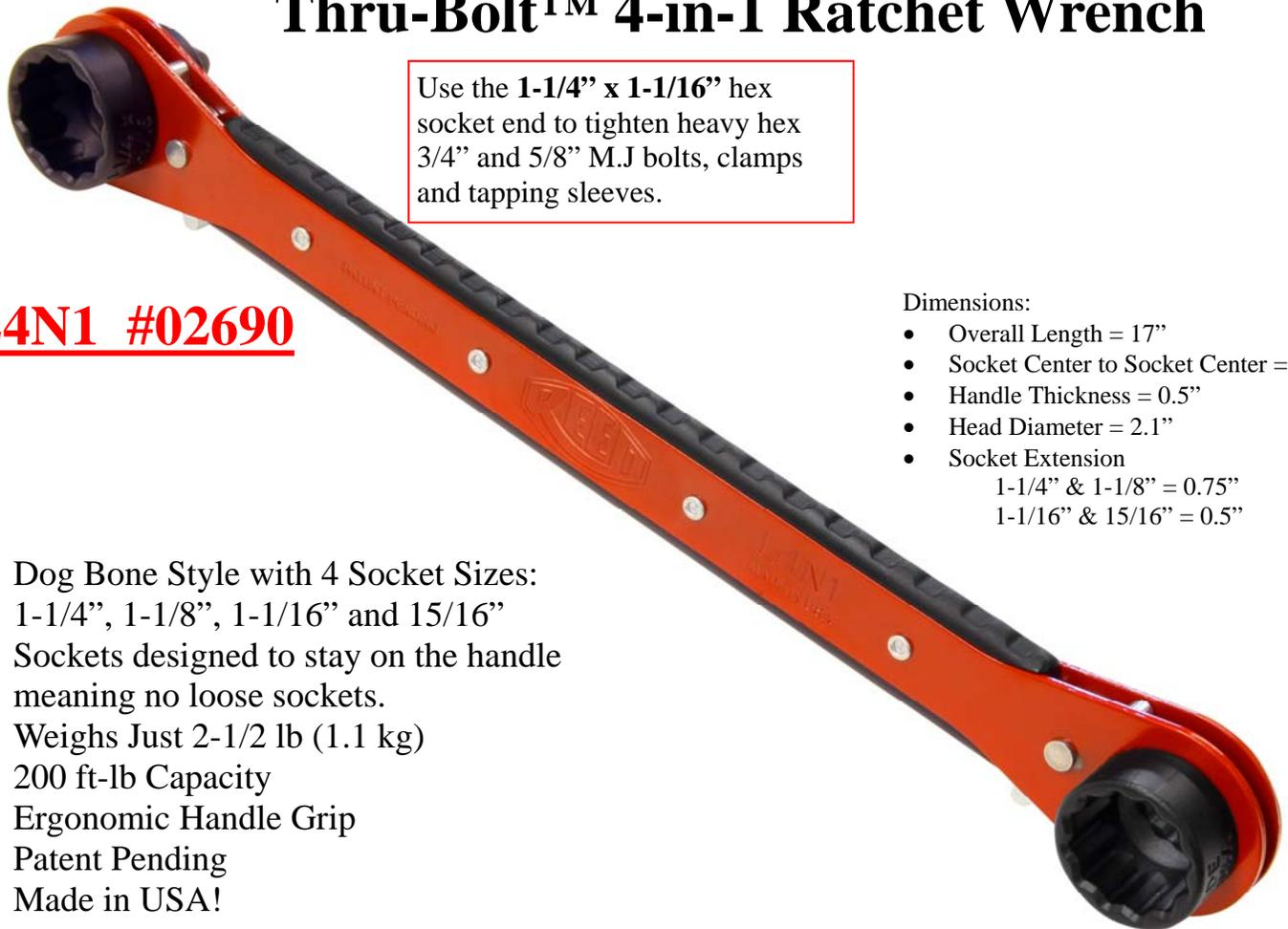
Use the 1-1/4" x 1-1/16" hex socket end to tighten heavy hex 3/4" and 5/8" M.J bolts, clamps and tapping sleeves.
