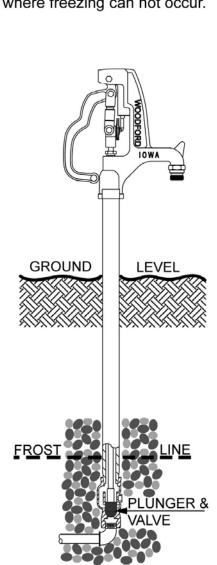
**OPEN - WATER FLOWING**Water flows when the handle is raised. The plunger is lifted allowing water to flow while sealing the drain hole.
